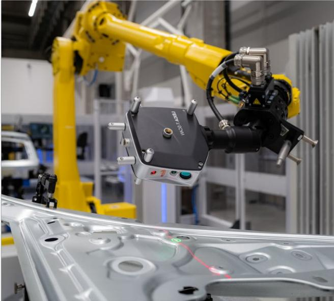
The system was designed to deliver the versatility ŠKODA AUTO needed, with an installed tool changer unit allowing for direct automated switching between high-speed scanning and more accurate tactile measurement. This variability means the system will always be able to perform measurement of difficult-to-access areas, such as openings, in a way that would simply not be possible for a less bespoke solution.
