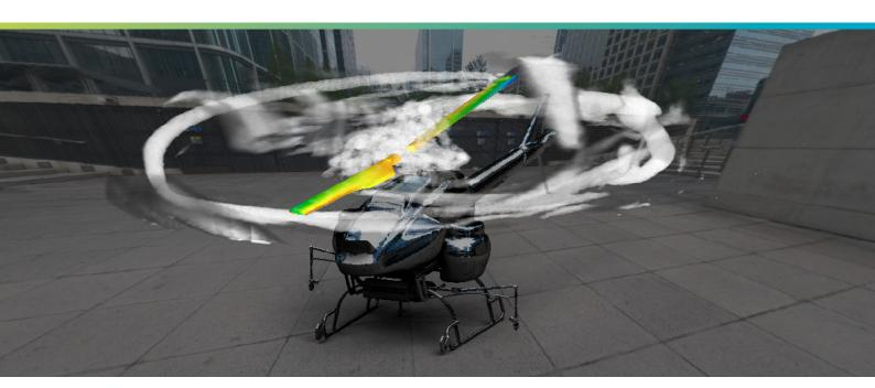
"The visualization of sound, which is invisible, has a great impact on the design development of an unmanned helicopter. We expect that effective co-simulation of a fluid analysis and a structural analysis will contribute to the development of high-performance tailor-made main rotors optimized for industry and usage."
