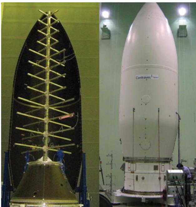
Figure 4: Vega Fairing at ESA ESTEC Large European Acoustic Facility during the Upper Composite Acoustic test
