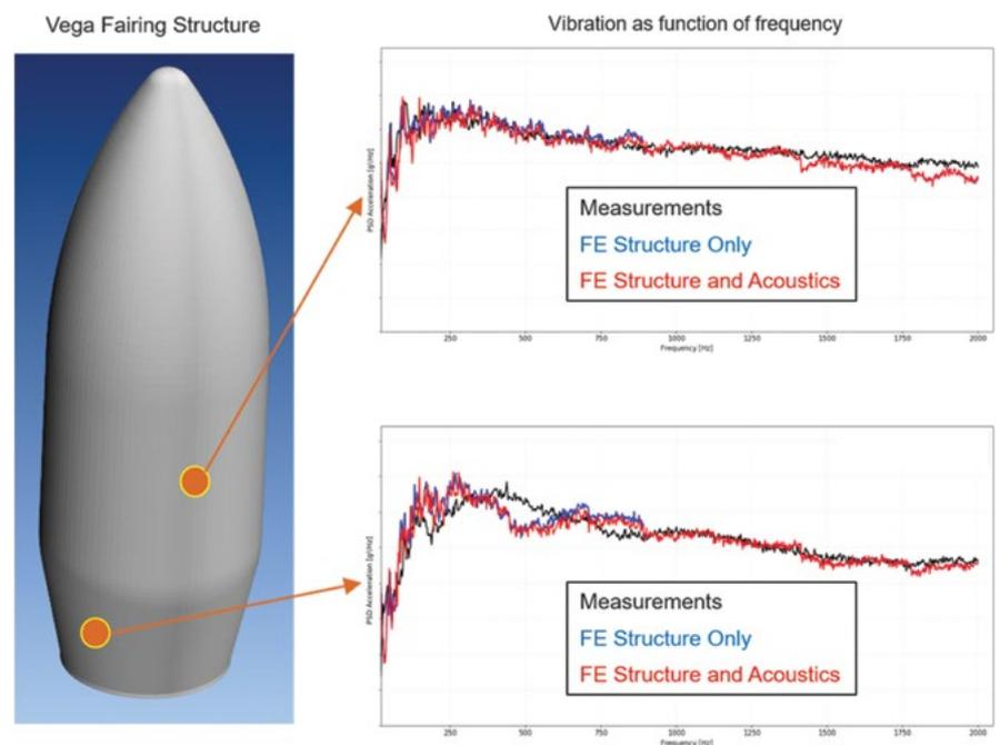
Figure 7: Vega Fairing - Vibration levels comparison
