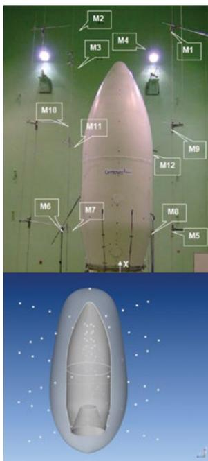
Figure 6: External and Internal acoustic domains with the relative microphones and measurement points.
