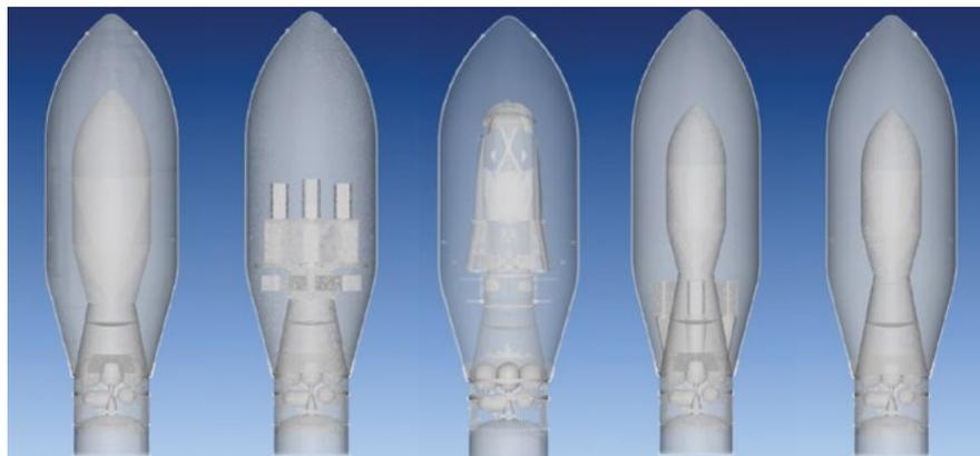
Figure 11: Vega C - Payloads configurations
