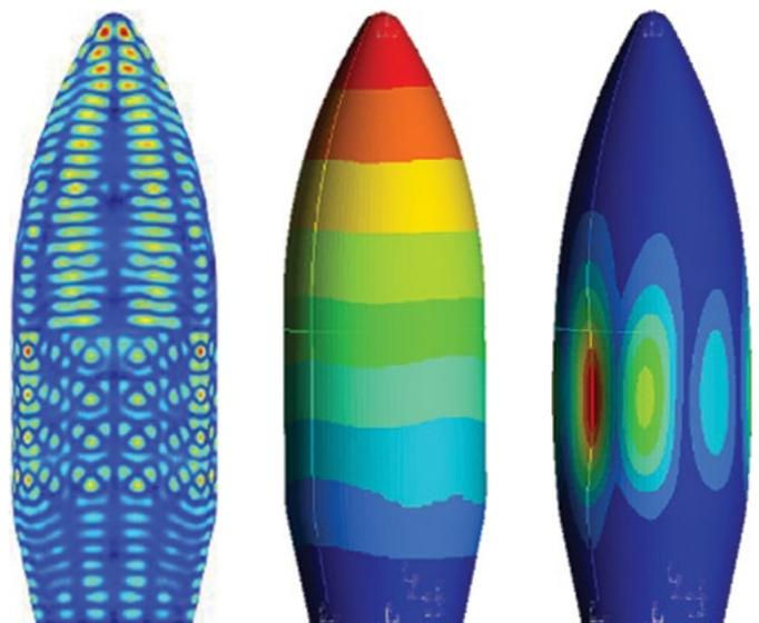
Figure 5: Eigenmode shapes extracted with MSC Nastran
