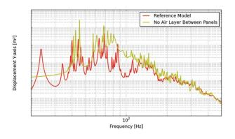
Figure 2. Solar Panels Vibration Spectrum, Impact of Air Interlayer Modeling
