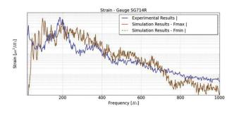
Figure 8. Solar Panel, Strain Power Spectrum
