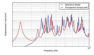
Figure 4. Solar Panels Vibration Spectrum, Impact of Panels Honeycomb Structure Modeling
