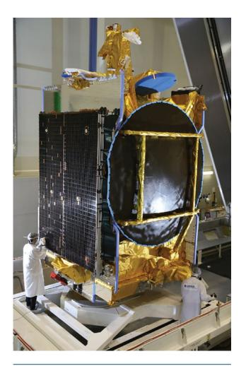
Figure 1. Telecommunication Satellite at IABG reverberation chamber, Copyright: Airbus Defence and Space 2017.
