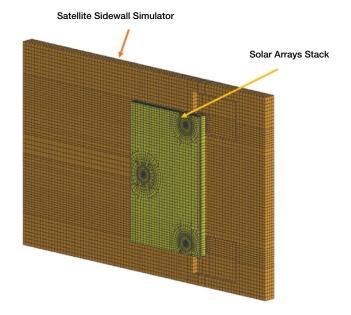
Figure 6. Vibro-Acoustic Model Overview
