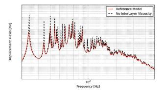
Figure 3. Solar Panels Vibration Spectrum, Impact of Panels Interlayer Viscosity Modeling
