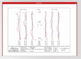
Due to the usually tight tolerances of globoid worms, only high precision 3D coordinate measuring machines with a small probing error P and scanning capability (i.e. Leitz PMM-C) should be used for such measurements.
