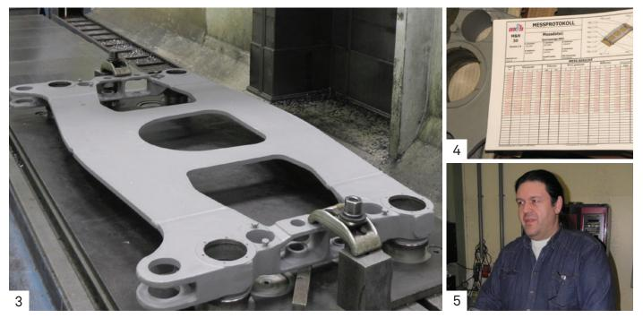
3| Undercarriage portals for bogieless tram cars are measured using m&h's 3D Form Inspect and finished to size
