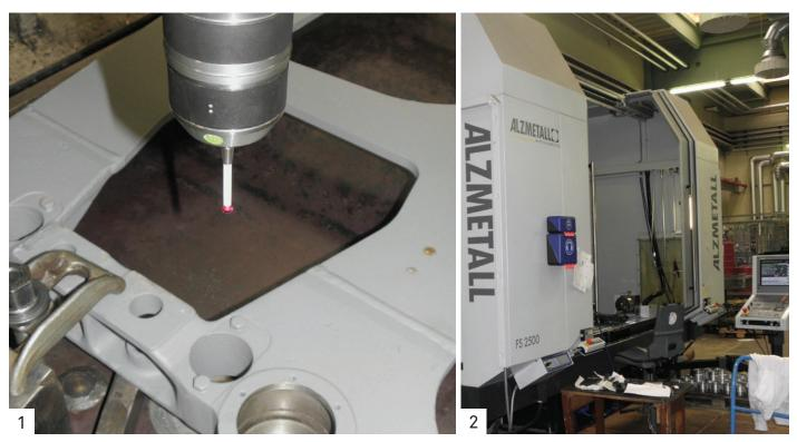
$|\ell|$  Measuring and machining of guide bushes on the machine are the key operations for the undercarriage portals
