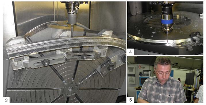
3| Milling, measuring and documenting curved surfaces directly in the machine tool at Dörr in St. Augustin. 4| Critical points between the machining steps can be checked at any time using 3D Form Inspect from m&h. 5| Roland Tillmann, head of fixture making, precision mechanics, contract manufacture and inspection gauges.
