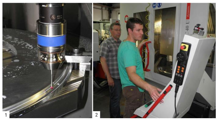
1| 3D Form Inspect makes it possible to check the nominal and actual geometry in the machine and, if necessary, immediately re-work in the same clamping arrangement. 2| With 3D Form Inspect the operator and supervisor always have an overview of the accuracy.
