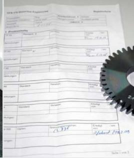
Why is steel subject to distortion during production? The scientists at the Bremen Institute for Metrology, Automation and Quality Science tackle this question by measuring 1,800 gear wheels using 3D measuring technology. The LSP-S2 probe takes data from each individual tooth, the faces and the holes.
