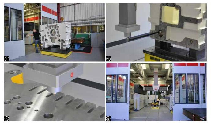
① Hexagon Metrology designed the entire Leitz PMM-G package: measuring machine and software, air-conditioned measuring room and feeding system. ② Optimum measurement precision is achieved even with long and heavy sensors. ③ Measuring a ram with the Leitz PMM-G. ④ The reinforced concrete base body ensures minimal mass movements.
