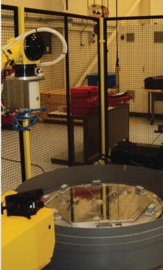
The race is on for who will manufacture 1,000 mirrors for the European Extremely Large Telescope (E-ELT). Cranfield University in the UK has begun work on producing seven of the mirror segments for 'the world's biggest eye on the sky' with the aid of high accuracy measurement systems from Hexagon Metrology.
