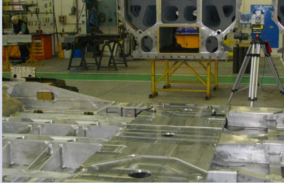
Semi-trailer chassis measuring more than 15 metres in length are measured using the Leica TDA5005.
