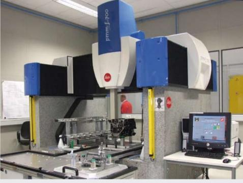
In 2002, PMM-F 700 started to be use at Audi. The process control is controlled by the quality guide lines.
