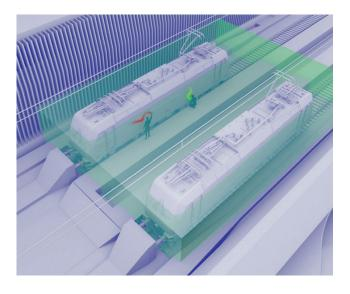
By placing a virtual security area around the parked wagons, vandalism of the wagons will be at a minimum. The lidars along
